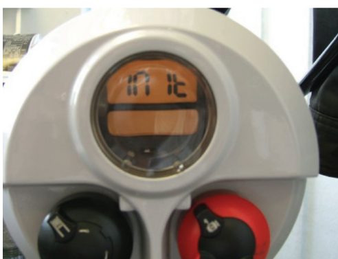
Commissioning mode initialised
