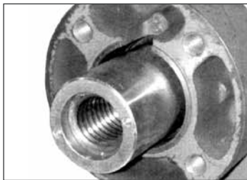
Fig. 4.11 Type Z3 Drive Bush in Position 3
