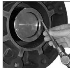
Fig. 4.6 Removal of Retainer
