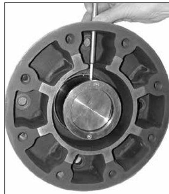
Fig. 4.12 Tightening Retainer Set Screw
