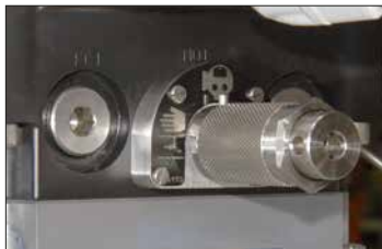
Fig. 6.1.1. Manual Override Handle
