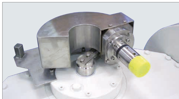
Position transducer assembly with electrical instrumentation connector.
