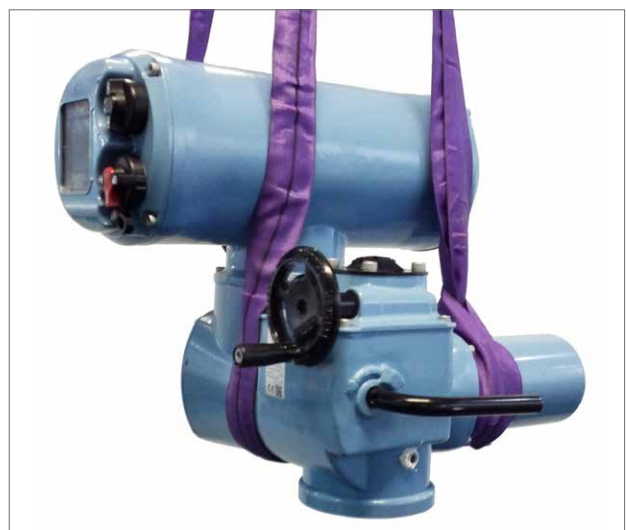
CK Centronik actuator being lifted in a sling.
