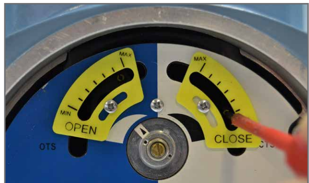
Close torque setting adjustment.
