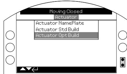
4. The Ethernet Option Card firmware version should be visible in the list. Please scroll down if the actuator has more options fitted; its type should be EtherNet/IP.
